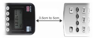
In very rare cases, the specified distance is too large. If the programming cannot be completed successfully, reduce the distance between the two remote controls and try it again.
