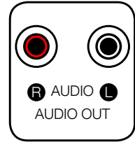
Example of RCA port
