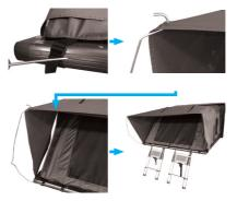
4. You can adjust the height using the rungs at the top. All rungs need to be fully extended and locked into place before use. When in use the ladder should be at
